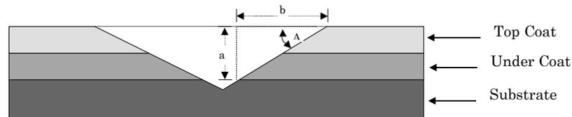
To find angle A using the formulas for the solutions of right-angled triangles,  $\tan A = a/b$ .
